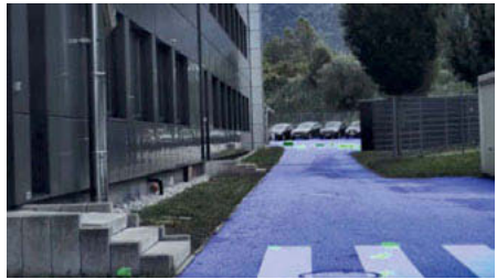
Figure 4: Result of a semantic segmentation with lost cargo marked in green.
