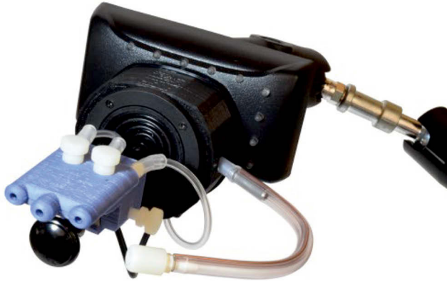
Figure 5 and 6: The QuadStick with pressure sensors for mouth control; Dennis Winkens' mouth control technique
