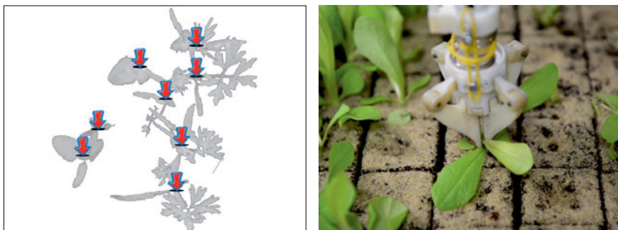
Figure 5.1: Field image with marked plant stem positions (left) and precision grasping of single plants based on stem position information (right).
