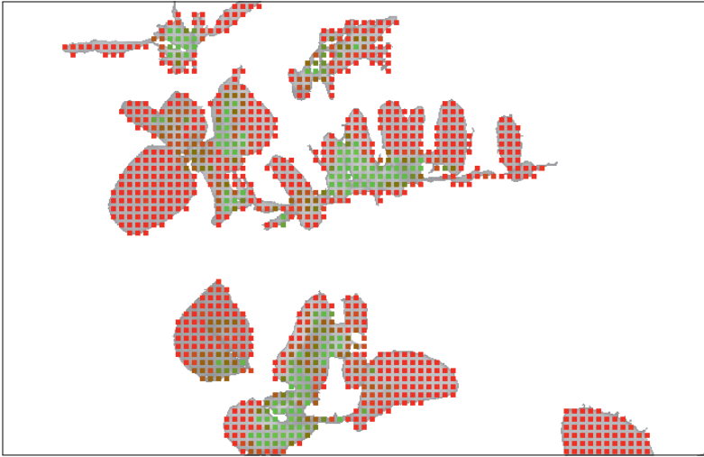
Figure 5.6: Stem certainty map in color code from red (i.e. no stem, s = 0 ) to green (i.e. stem, s = 1 ). The scores are plotted at the corresponding keypoints.
