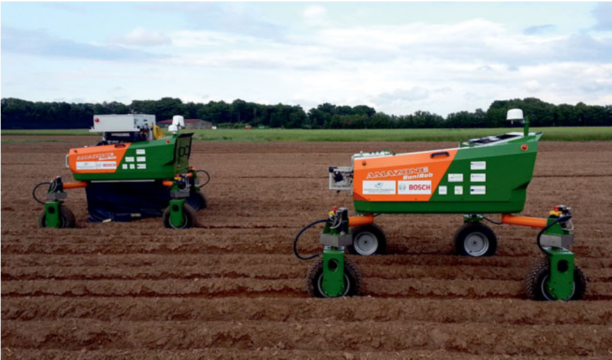
Figure 6.1: Two BoniRob V2 robots in a field: The robot has free space inside which can be used to mount an app module (right robot). The sensing and plant classification and position estimation system developed in this thesis is mounted in the left robot.
