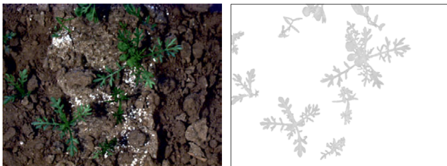
Figure 3.1: Sample image (color channel, left) and result of vegetation segmentation (right). These images are produced by the camera system and segmentation method which are discussed in this chapter.
