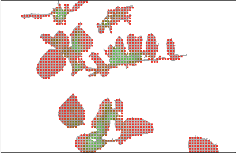
Figure 5.7: Filtered stem certainty map in color code from red (no stem) to green (stem). The image is the same as in Figure 5.6.
