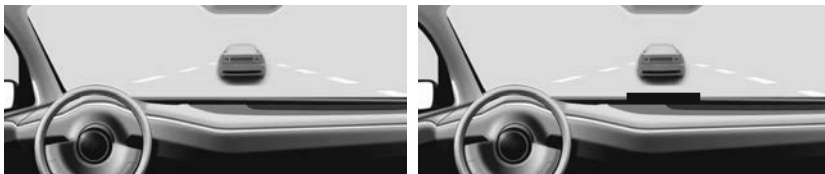
Fig. 1: Design of condition “Basic SAE2 indication” blue sides and orange in front (left) and design of “Basic SAE2 indication + detected object” blue sides and orange with blue bar in front (right)
