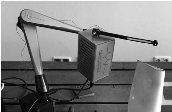
Fig. 3: Scalable automatic modal hammer (SAM) in operation, built on a hydraulic arm with magnetic stand. The impact point is set at the back side of the trailing edge tip of the blade and results in an impulse of the out-of-plane direction.
