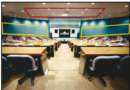
Figure 27. Typical SPAS presentation room, with ACT ceiling and carpeted floor. Suggested reflective, diffusive and absorptive treatment areas are outlined in blue, yellow and red.
