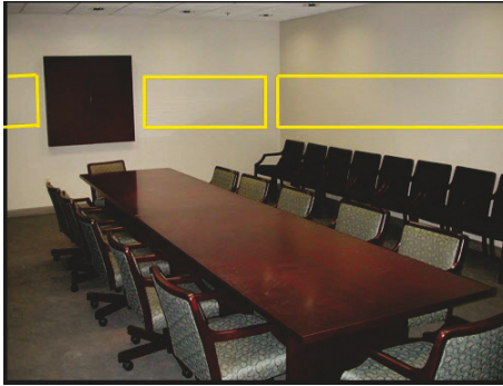
Figure 25. Typical SPAS meeting room design, high frequency absorption on ceiling (ACT) and floor (carpeting) and no absorption on walls. Yellow rectangles indicate area for diffusive treatment.
