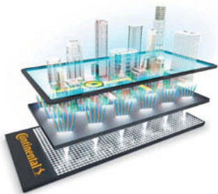
Fig. 2: Functional principle 3D backlighting
