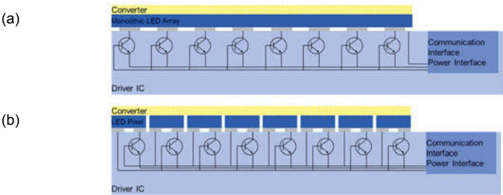
Fig. 1: Schematic cross section of different HDSSL light sources with (a) monolithic and (b) separated LED pixels carried by a Driver IC (ASIC)
