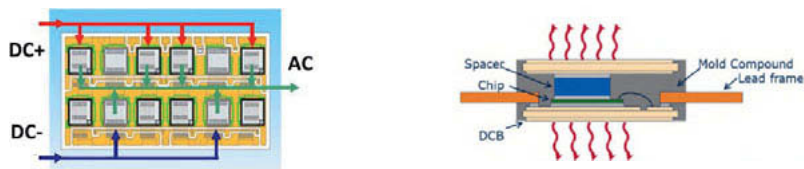
Fig. 2: Traditional Low stray inductive designs: left to right: Bondwire DBC, Direct lead bond
