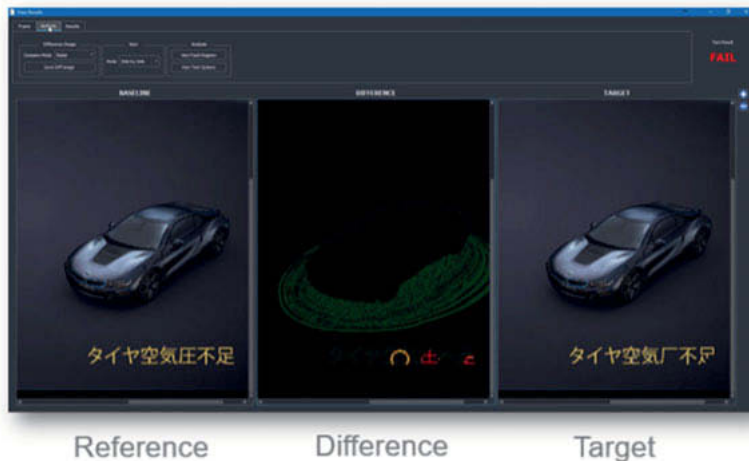
Fig. 3: In an Altia Automated Test, the reference design is compared with the design on target. Differences are shown in a heat map format – green for minor differences, yellow for more significant differences and red for severe differences.
