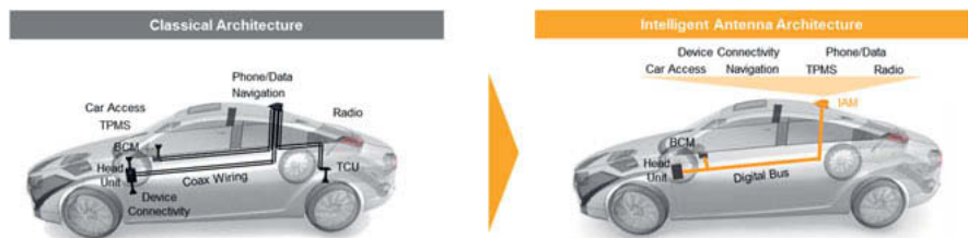
Fig. 4: Comparison between classical and IAM architecture
