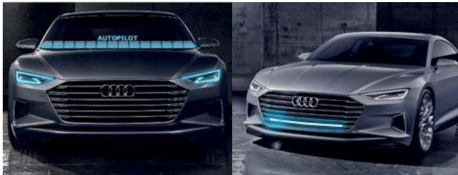
Fig. 2: Possible lighting signals in the windshield and in the front, but what is the meaning of the signals? Is it the right color? Is it the right wording?
