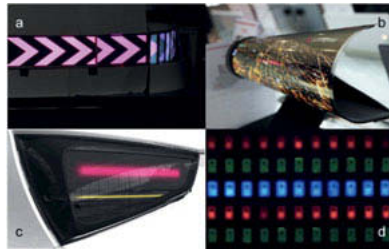
Fig. 2: Display technologies for automotive signal applications: a) LCD, b) AMOLED [6] c) LED matrix, d) Micro-LED [9]
