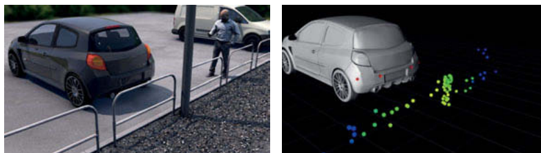
Fig. 1: Ultrasonic perception for automobiles (animation)
