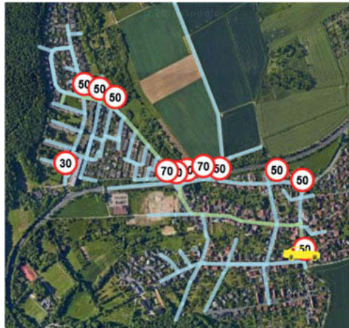
Fig. 4: Visualization of an exemplary horizon containing speed limits
