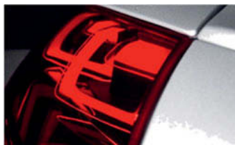
Fig. 9: Principle illustration, flexible OLED following curvature of car shape and lamp curvature of AUDI TT
