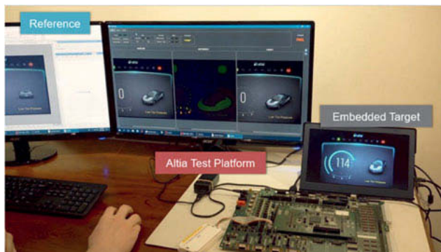
Fig. 3: An example of an Altia Automated Test setup. A custom hardware-software capture rig (off screen) compares the reference design GUI (left) to the GUI on the embedded target (right). Differences found during test are displayed on the screen in the center of this setup.
