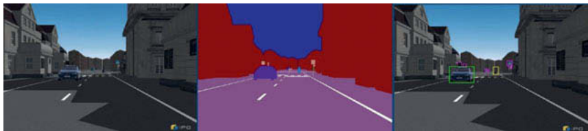
Fig. 1: Synthetically generated image (left), pixel-accurate semantic segmentation (center) bounding box annotation (right)
