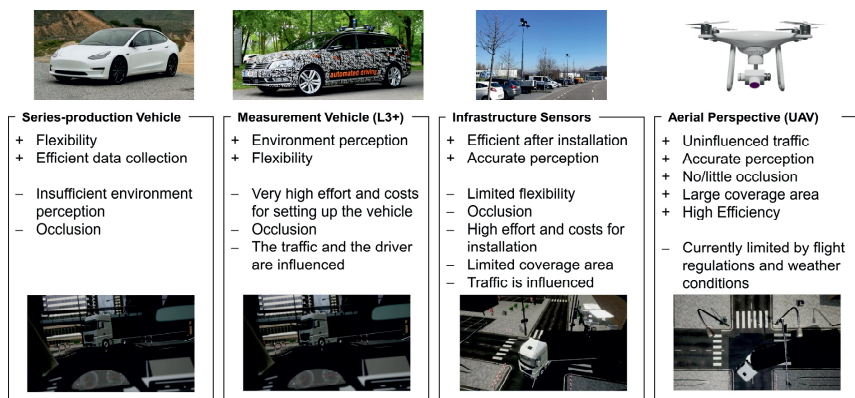
Fig. 2: Comparison of four measurement methods for trajectory dataset generation. Series-production vehicles, measurement vehicles equipped with reference systems, infrastructure sensors and the aerial perspective representing the drone-based method.
