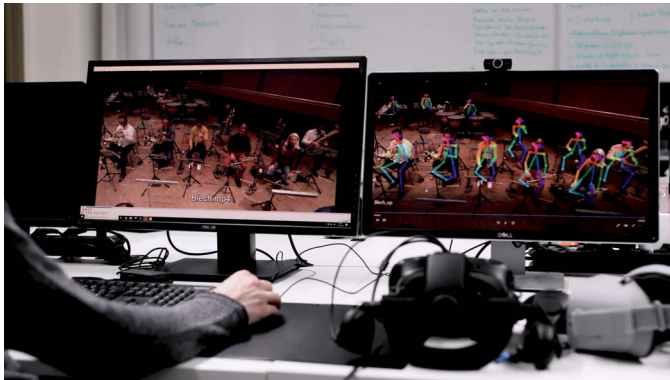
Figure 4: Real-time prototype for visualizing the skeleton joint positions of a musicians superimposed on top of an image of the real persons.
