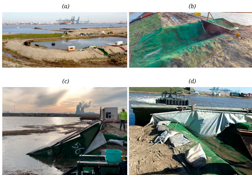
Figure 11.5. (a) The purposely build test facility in the former Hedwigepolder. (b) Artificial breach with hatch for BresDefender experiments. (c) Pontoon covered with flexible sheet placed in front of breach. (d) Flow reduction through breach after application of pontoon. All images from February/March 2022. Figure source: Bureau Multimedia, Den Helder.
