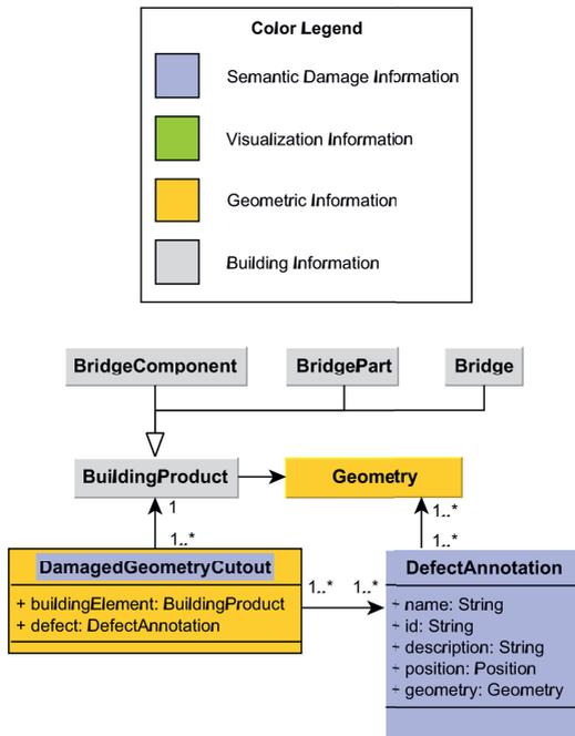
Figure 3.14: Class diagram for modeling the damaged component geometry with the component geometry and the defect geometry. The relationship *DamagedGeometryCutout* influences the geometry, hence, it is colored in blue and yellow.
