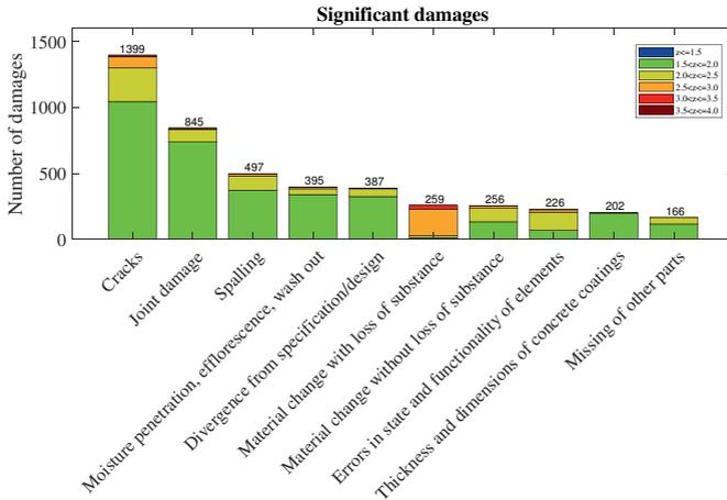
Figure 3.7: Top ten most severe defects at bridges in Thuringia, Germany, considering the severity. The colors display the Z-rating between one and four [12].
