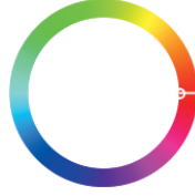
Figure 2.4: Color coding of the orientation of the estimated velocities. Orientations are relative to the current orientation of the robot (white mark to the right).
