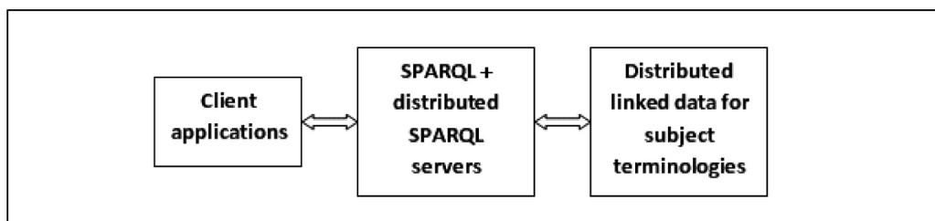
Figure 2. Distributed architecture base on the semantic web
