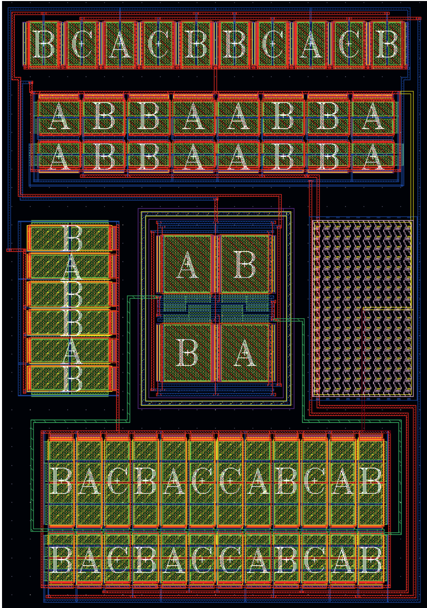
Figure 4.20: Finalized layout of the Folded Cascode OTA, obtained by SWARM for a 2:3 aspect ratio.
