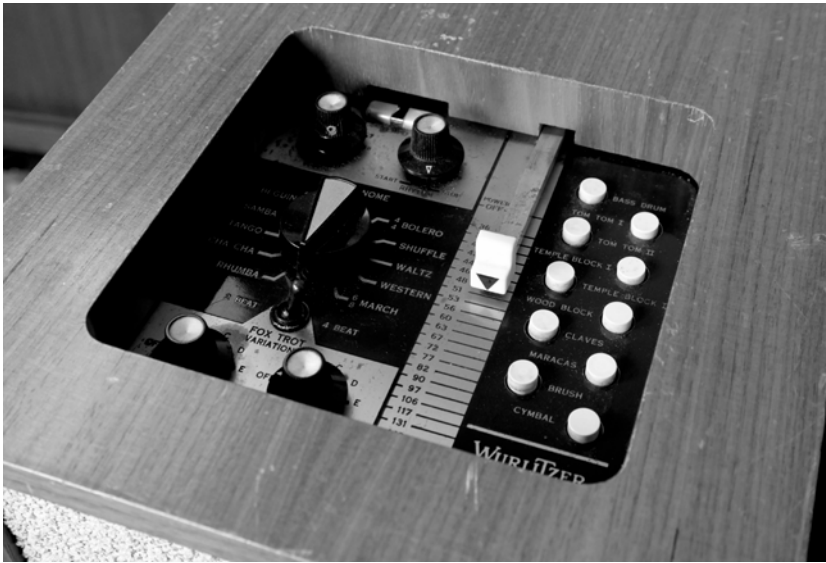
Figure 3: Wurlitzer Sideman. Panel for controlling volume, start-stop, patterns and variations, and tempo, along with buttons to play individual sounds. Photo: Robert Michler, 2022
