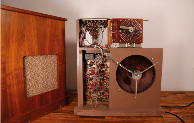
Figure 2: The electro-mechanical construction with hand-wired connections, a constantly rotating disc to set a steady tempo, and a connected comb to pick up signals at the contact points created the different grooves. This principle was unique and very different to subsequent drum machines. Thus, its key features were seminal with regard to the preset patterns included. Photo: Robert Michler, 2022
