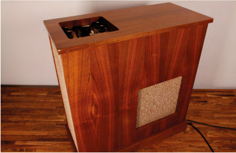
Figure 1: The Wurlitzer Sideman came in a heavy wooden box. It included an integrated amplifier and internal tubes, resulting in a total weight of approximately 40 kg. Photo: Robert Michler, 2022
