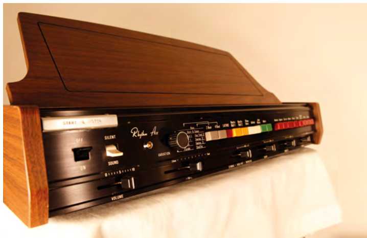
Figure 4: The Bentley Rhythm Ace FR-8L drum machine – with a nearly identical construction to the Roland TR-77 20 and similar to other models – was designed for use by organ, keyboard, or guitar performers: The flatter form made it possible to lay the device on top of the instrument, while the note stand was designed to fold out. Apart from the usual knobs used to select patterns and combinations, individual instruments had their own volume fader, thereby enabling the preset’s character to be changed. The start-stop button, located in the top left corner of the panel, was built as a touch-sensitive metal-retainer. Photo: Robert Michler, 2022
