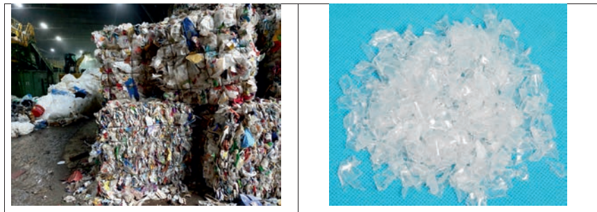
Fig. 8: Bales of mixed, contaminated waste (left) were divided into individual fractions and processed into mono-material flakes (right) - here taking the example of PET.
