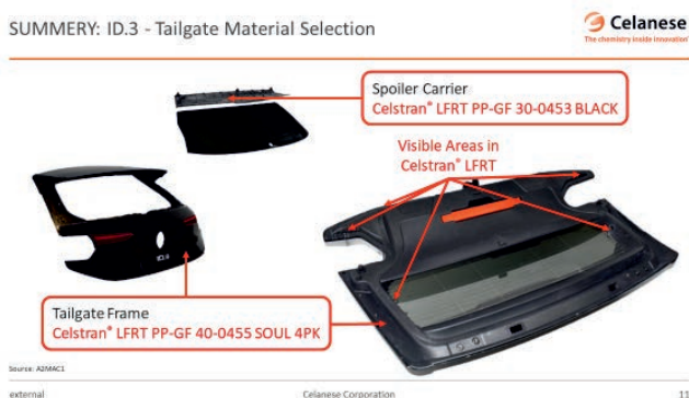
Fig. 7: Material selection for the tailgate frame and spoiler carrier
