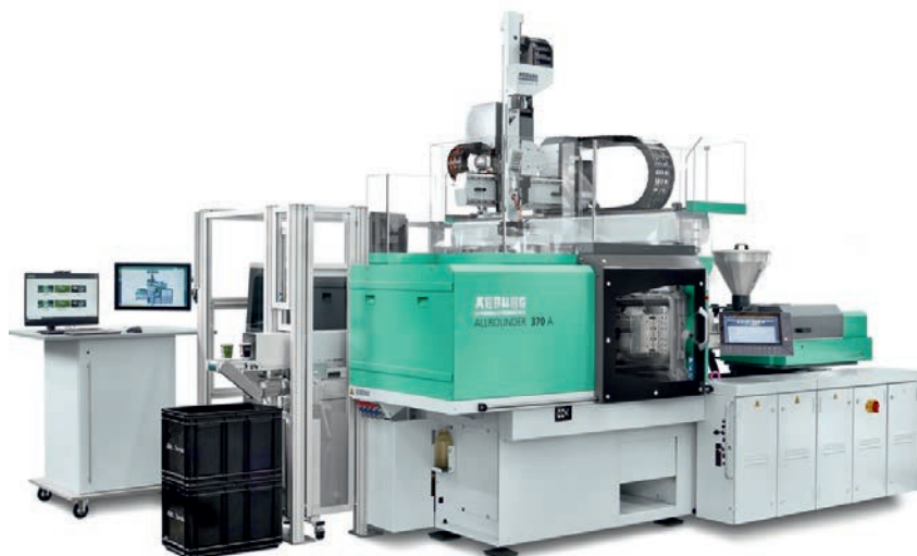
Fig. 2: Arburg turnkey system for sustainable reusable cups
