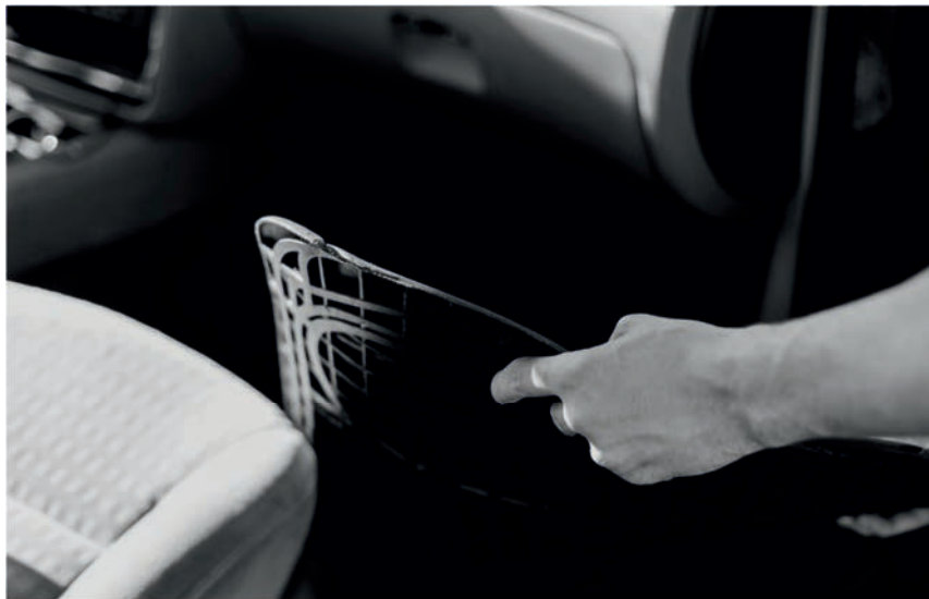
Fig. 1: All-weather floormat made from TPE [1]
