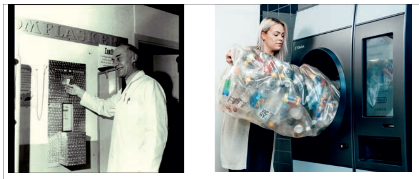
Fig. 2: The first deposit machine, the Tomra 1A (left) from 1972 (with photocells and halogen lamps), and the latest development (right), the Tomra R1 from 2020.
