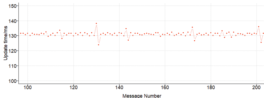
Figure 8: Excerpt of update time sequence chart of TC02 (FTT 5G, DL, TI = 131 ms) downlink.
